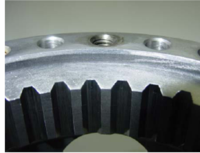
CHAMFERED FACE ON END OF SPLINES
